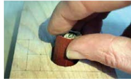
Drilling can burnish the inside of the hole so key it up with some coarse abrasive
