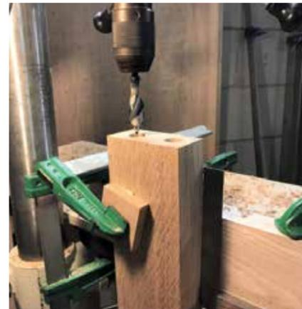
Use a fence attached to the drill table to square the component up for drilling
