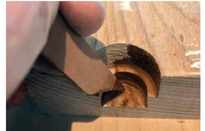
Use a basic resin to completely wet out the hole
